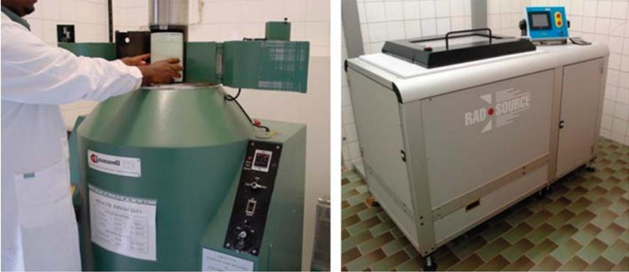
FIG. F.4. Gamma ray (left) or X ray (right) irradiators are used for sterilization of male mosquitoes.
