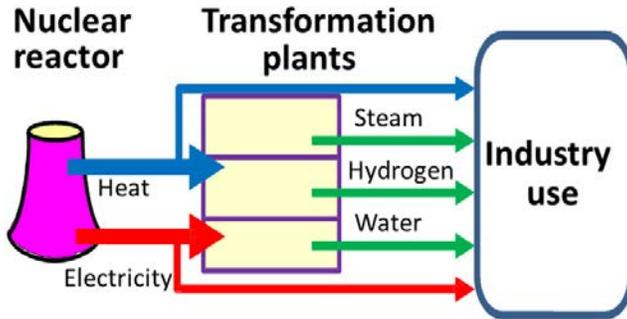
FIG. B.5. General scheme for coupling a nuclear reactor to an on-site industrial plant.
