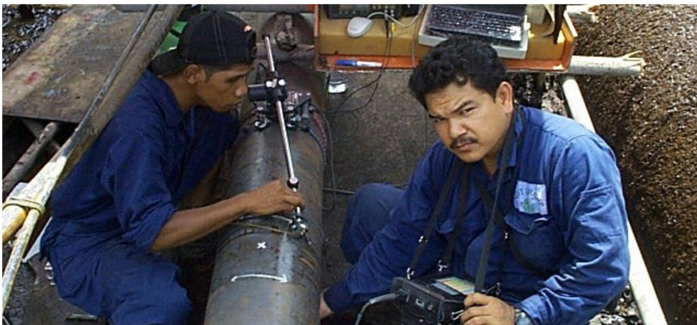
Technicians inspecting a PETRONAS pipe using NDT methods in order to test the quality of the pipeline.
