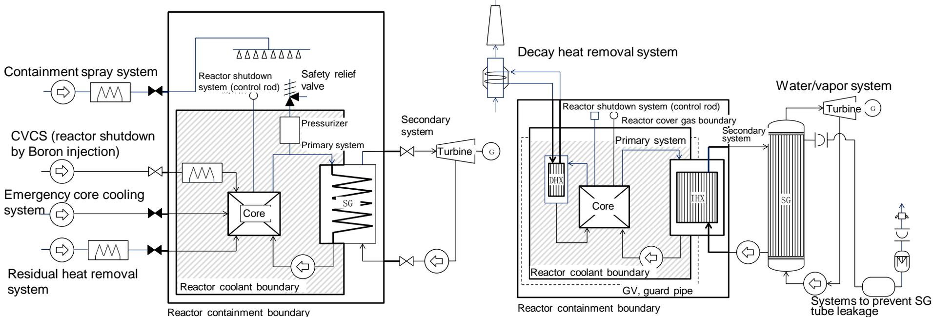
**Concept for cooling system for PWR**
