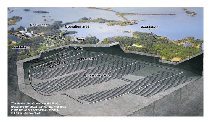
power. In every option, deep geological disposal is the preferred final end point. The principle of geological disposal is to isolate the waste deep inside a suitable host formation, e.g. granite, salt or clay. The waste is placed in an underground facility or disposal facility, designed to ensure that a system of natural and multiple artificial barriers work together to prevent radioactivity from escaping.
