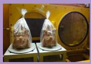
Through a coordinated research project, the IAEA Physics Section supported the development of large sample neutron activation analysis as the only existing method to measure non-destructively the bulk mass fractions of the elements present in samples up to kilograms in mass. Examples include archaeological artefacts, excavated rock samples, large samples of assorted ore, and nuclear reactor components. More information at https://nucleus\_iaea.org/rrdb/
