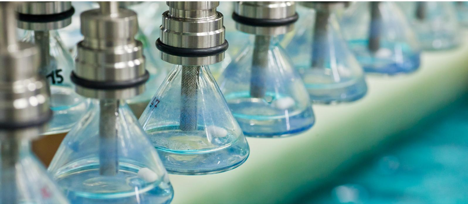
Oxygen isotope fingerprints of water give information about its origin and age, and they are measured by equilibrating water samples with CO<sub>2</sub> gas in the laboratory using mass spectrometry. (Photo: IAEA)
