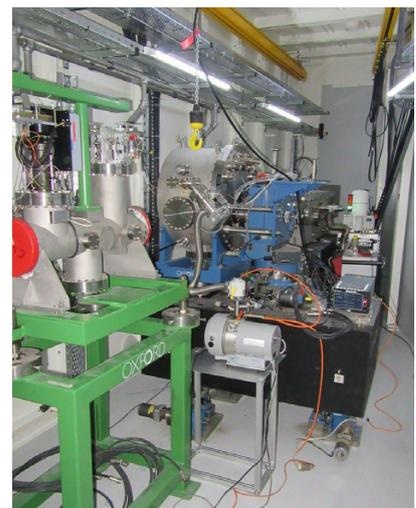
Typical example of a 1.7 MV tandem accelerator facility
