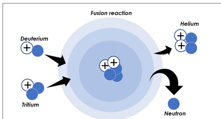
**A mixture of Deuterium and Tritium — two Hydrogen isotopes — will be used to fuel future fusion power plants. Inside the reactor, Deuterium and Tritium nuclei collide and fuse, releasing Helium and neutrons.**
