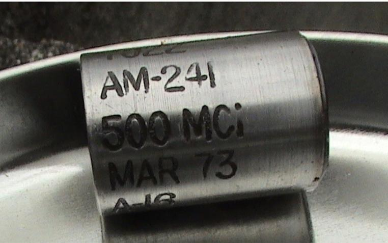
**Sealed radioactive sources consist of radioactive materials isolated from the environment in a sealed metal capsule.**
