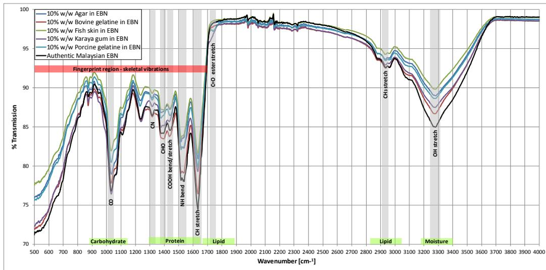
FIG. 6: The infrared % transmission spectra (4000 to 500  $\text{cm}^{-1}$ ) obtained from an authentic Malaysian EBN using mid-infrared spectroscopy with attenuated total reflectance micro-diamond sampling adapter. The figure also shows the spectra obtained for common structural adulterants at 10% (w/w) in EBN and the absorption bands for a range of functional groups
