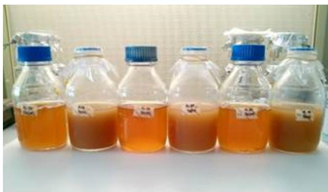
FIG. 8: Aerobic (bottles with plastic covers) growth was faster than anaerobic growth (bottles with blue caps), leading to greater yields as evidenced through higher optical density values and pallet size
