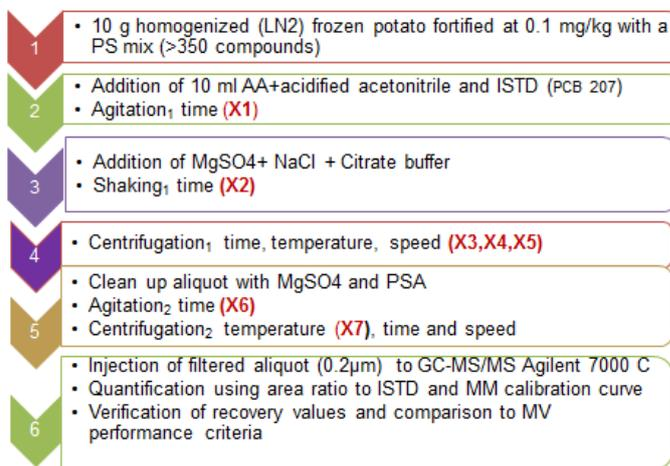
FIG. 10: The method used and the X factors
