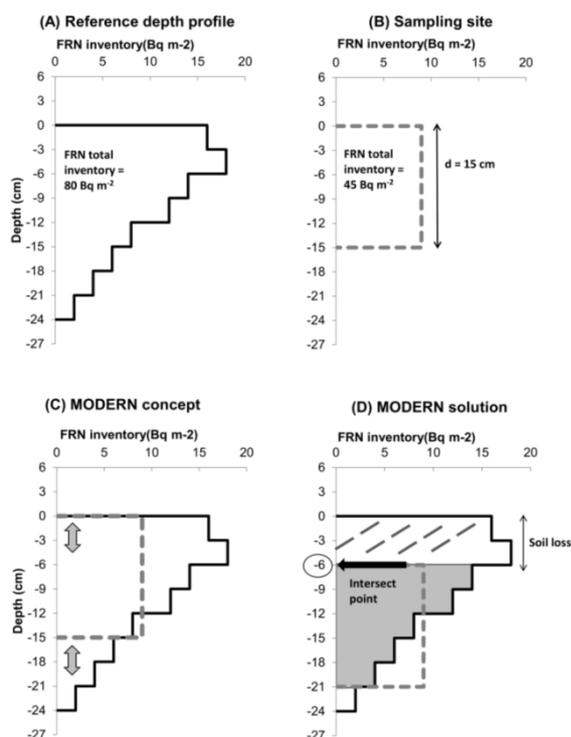
FIG. 1: Concept of the conversion model MODERN (Modelling Deposition and Erosion rates with Radionuclides)
