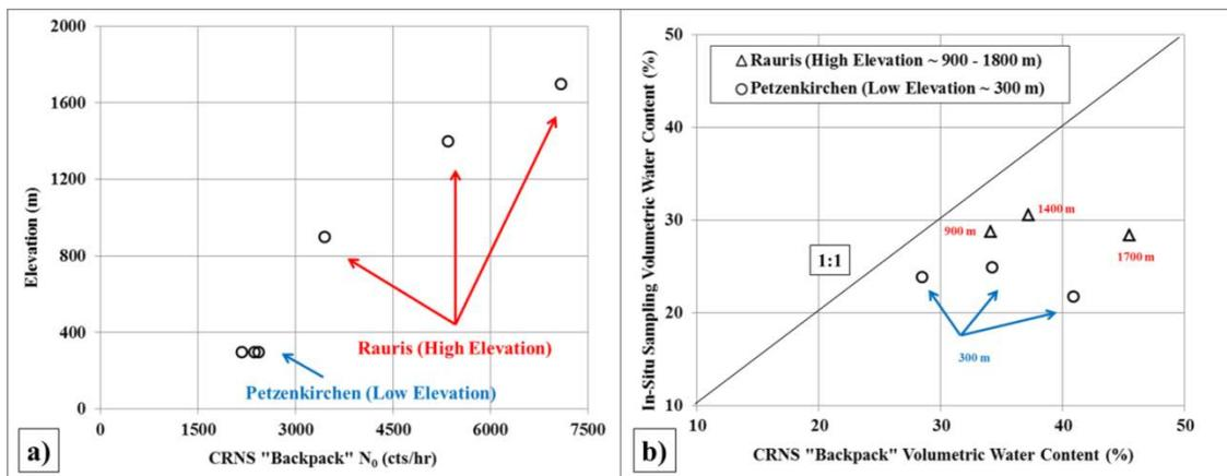
FIG. 11: a) CRNS ‘backpack’ cosmic ray neutron counts per hour (cts/hr) is compared to elevation across three field sites located at different elevations near Rauris, Austria, and a low elevation site near Petzenkirchen, Austria. b) Comparison of SWC values determined via the CRNS ‘backpack’ and traditional *in-situ* sampling of SWC across all four field study sites (high and low elevations)
