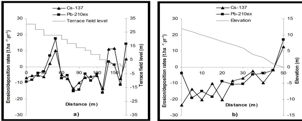
FIG. 3: Soil redistribution rates along a) the terraced field and b) the unprotected field
