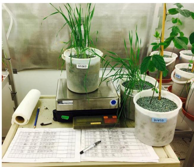
FIG. 5: Daily gravimetric analysis. The pot surface is covered with blue plastic beads to minimize soil evaporation.
