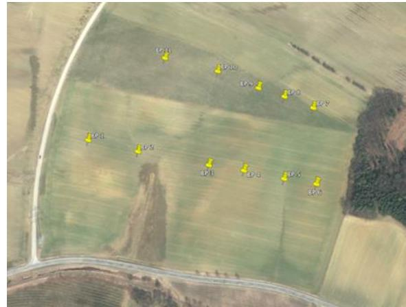
FIG. 9: Location of 11 backpack survey points collected on 6th of July 2017 in Grabenegg Austria. The backpack was left at each location for ~15 minutes. A mobile TDR sensor (0-15 cm) was used at ten locations around each backpack survey point. The TDR system was only used on the first six survey points due to challenging soil conditions
