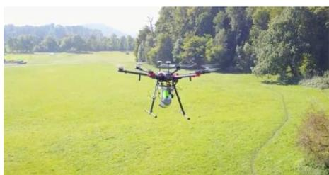
FIG. 12: Field test of a drone equipped with a mosquito release device
