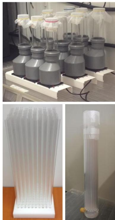
FIG. 11: Various systems developed to measure mosquito flight ability. Top, aspirator device used to impose an aspiration stress exposure to mosquitoes; bottom left, 40 cm high flight organ device used to test the quality of adults emerging from pupae; bottom right, flight organ device used to test the quality directly of adults
