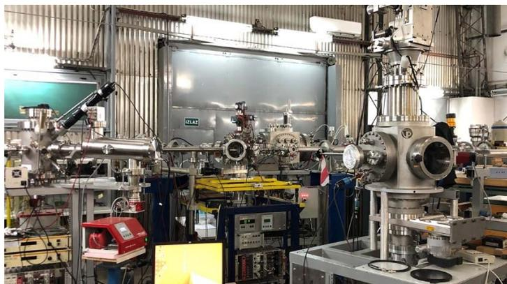
FIG. C-1. L'installation He Ion Source & DiFU Dual-Beam à l'Institut Ruđer Bošković, en Croatie.
