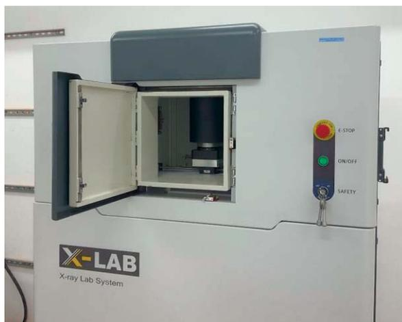
**FIG. 6:** Nuctech X-Lab prototype twin horizontal beam X-ray irradiator © A.G. Parker
