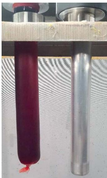
**FIG. 11:** Sausage heating device developed at the IPCL to reduce the amount of blood necessary to feed a mass-rearing cage.
