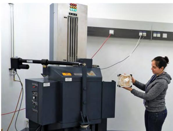
FIG. 17. Ms Paloma Guazzelli Della Giustine, a fellow from Brazil performing irradiation experiments to determine irradiation dose-response curves for *Anastrepha fraterculus*
