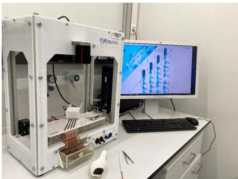
*FIG. 5. The Near InfraRed Pupae Sex Sorter (NIRPSS) and the images obtained as displayed on the computer screen*
