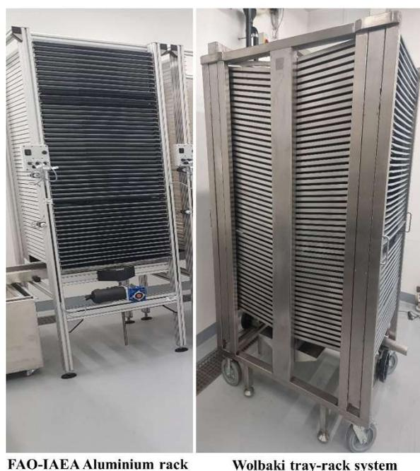
FIG. 11. The FAO/IAEA (left) and Wolbaki (right) rearing rack systems.
