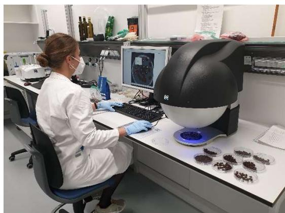
*Multispectral imaging MSI analysis of Arabica and Robusta coffee at FEPL.*
