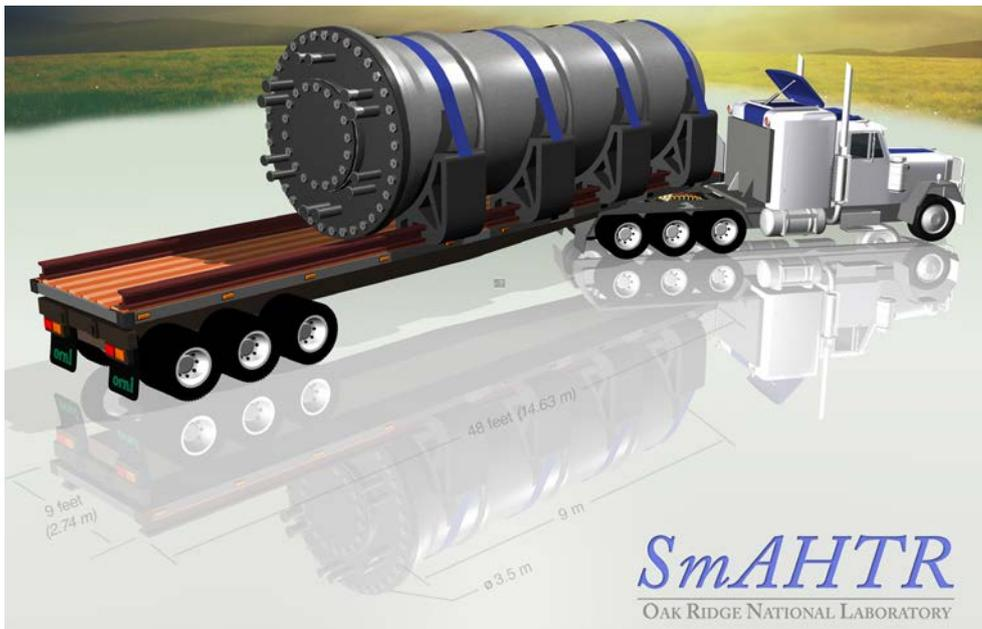
**Many SMR reactors are designed to be small enough to be transported by truck or shipping container.**
