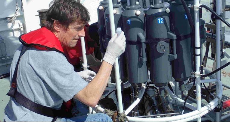
**A scientist from the IAEA Environment Laboratories takes samples of seawater to study the role of microbes in the ocean carbon cycle.** (Photo: R. Hansman/IAEA)
