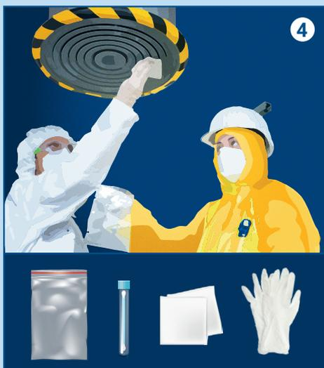
④ **Environmental swipe sample kits** may be used to take samples of dust that can reveal the presence of nuclear material particles. If found, these particles can indicate if any undeclared nuclear activities have taken place (see page 10).
