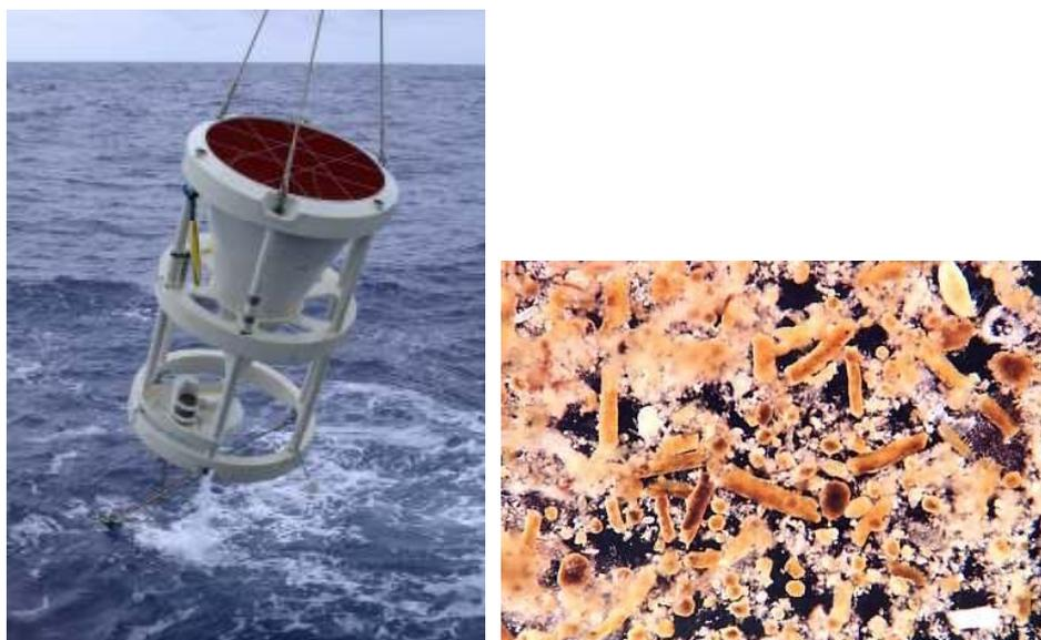
*FIG. 5 Sediment trap (left) used to catch marine particles (right) that settle from the surface to the deep ocean.*
