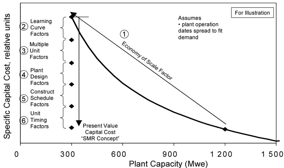
FIG. 6. A generic scheme illustrating potential SMR economic factor advantages (courtesy of Westinghouse, USA).
