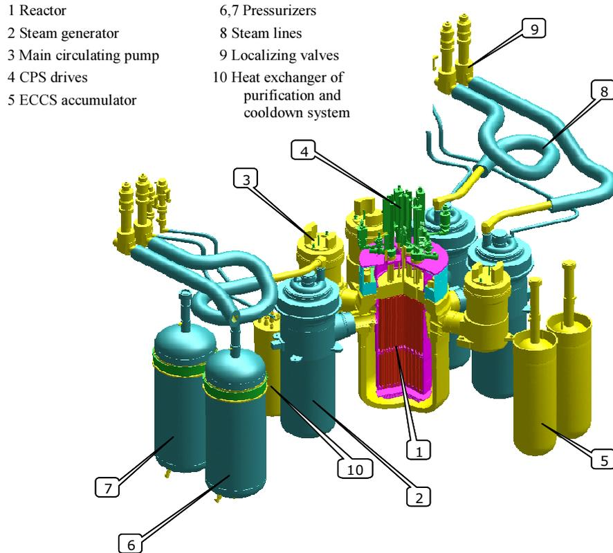
FIG. 2. Modular layout of the KLT-40S reactor plant (Source: OKBM, Russian Federation).
