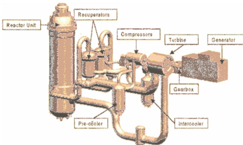
FIG. 3. Conceptual layout of the PBMR primary system, offering >41% energy conversion efficiency with direct gas turbine cycle (Source: PBMR Ltd., South Africa).
