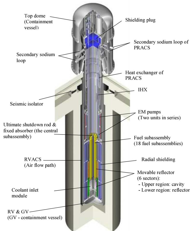
FIG. 5. General view of the 4S sodium cooled reactor with a 10 – 30-year refuelling interval for a 50 MW(e) plant (Toshiba – CRIEPI, Japan)
