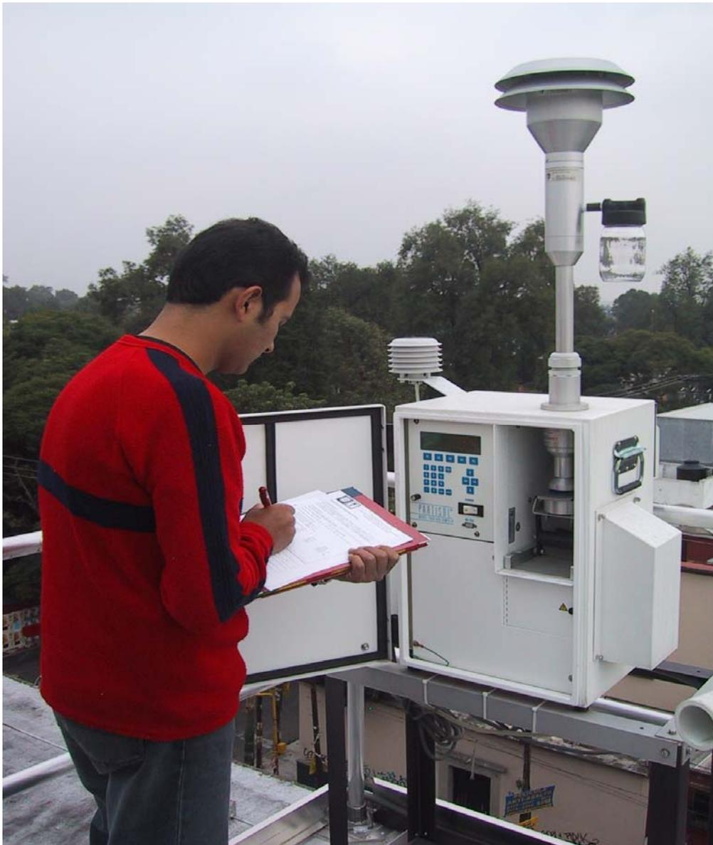
*FIG. 11. A technician collects current operational data from the fine particle air sampler at the atmospheric sampling site at Coyoacán, in the greater metropolitan area of Mexico City. (Photo courtesy of the National Nuclear Research Institute, Mexico.)*
