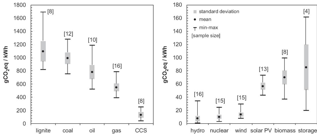
FIG. VII-3. Summary of life-cycle GHG emissions for selected power generation technologies<sup>9</sup>.
