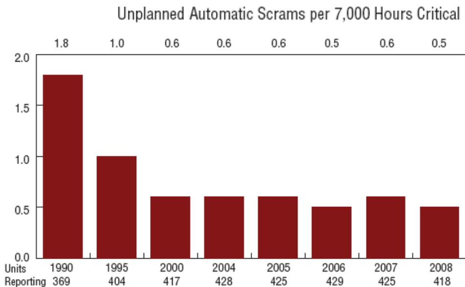
Figure 3: Unplanned automatic scrams per 7000 hours critical (source: 2008 Performance Indicators World Association of Nuclear Operators)
