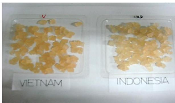
Cassava starch+KOH+Acrylic Acid after irradiation and dried in preparation of super water absorbent.
