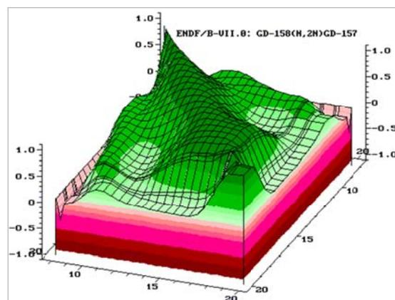
FIG. C-1. Three-dimensional plot of energy–energy correlations for nuclear reaction cross sections.
