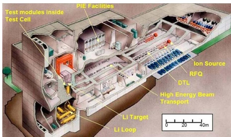
FIG. C-2. Conceptual design of IFMIF (PIE = post-irradiation examination; RFQ = radio frequency quadrupole; DTL = drift tube linac).
