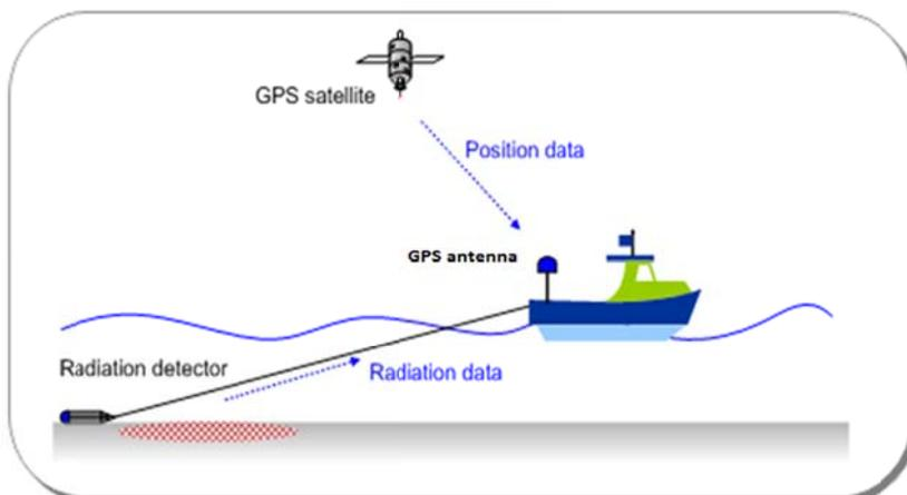
FIG. I-2. Sketch of GPS integrated gamma counting system for sediment tracing studies in a coastal area.
