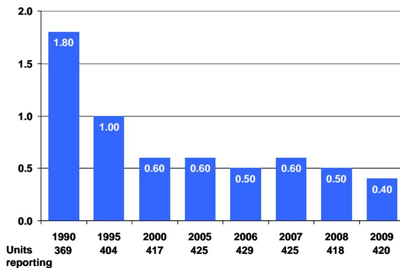
FIG. A-3. Unplanned automatic scrams per 7000 hours critical (source: WANO 2009 Performance Indicators).
