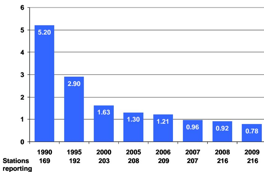
FIG. A-4. Industrial safety accident rate at nuclear power plants — number per 1 000 000 person-hours worked (source: WANO 2009 Performance Indicators). Note: These incidents are not necessarily radiological in nature.
