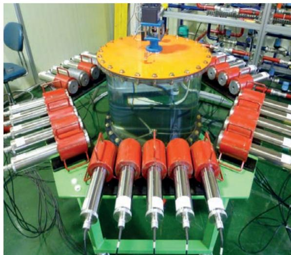
FIG. 3. Industrial single photon emission computed tomography system for the radiotracer visualization of  $^{68}\text{Ga}$  and  $^{137\text{m}}\text{Ba}$  from generators.
