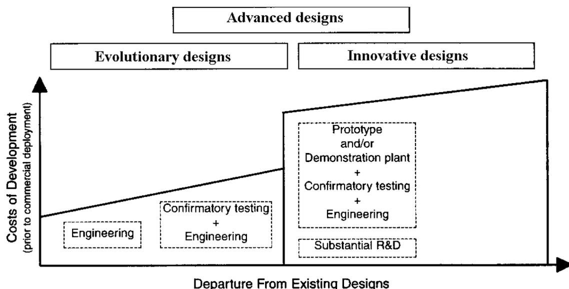
FIG. IV-1. Classification of advanced reactor designs.
