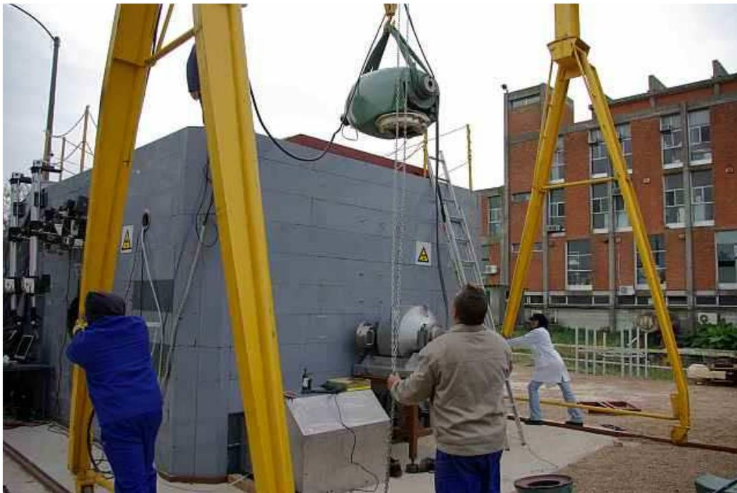
FIG. VI-6. The mobile hot cell in operation in Uruguay.
