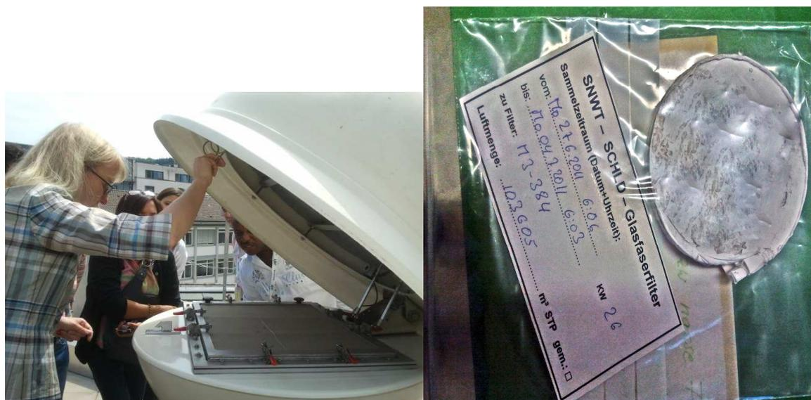
*FIG. F.1. Large volume aerosol collector operated by the Federal Office for Radiation Protection in Salzgitter, Germany, and aerosol filter compacted for immediate gamma spectrometric counting - being demonstrated to participants in the Agency's Interregional Advanced Training Course on Marine Radioactivity: Analytical Techniques and Quality Management hosted by the Karlsruhe Institute of Technology in 2011.*
