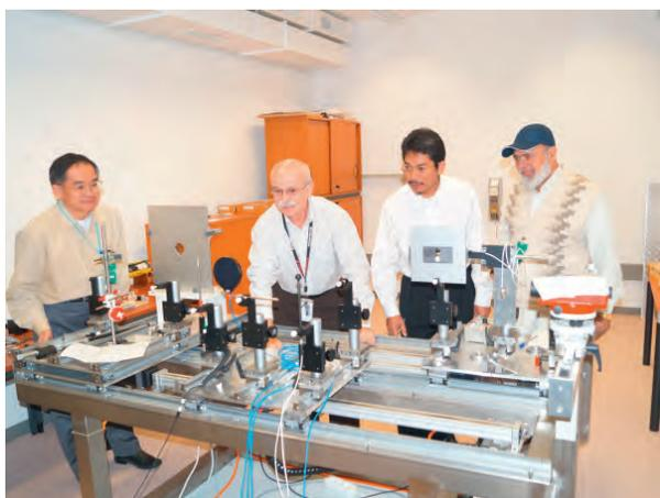
FIG. 2. Comparison measurements of national dosimetry standards in X ray beams during a technical meeting at the Agency's Dosimetry Laboratory in Seibersdorf.
