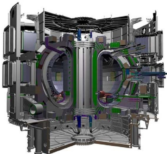
*FIG. B-2. Cutaway view of the ITER device which is being built in France to investigate fusion energy production. Extensive amounts of nuclear and atomic data have been used in the design of the device and will be used to analyse its operation and experiments.*
