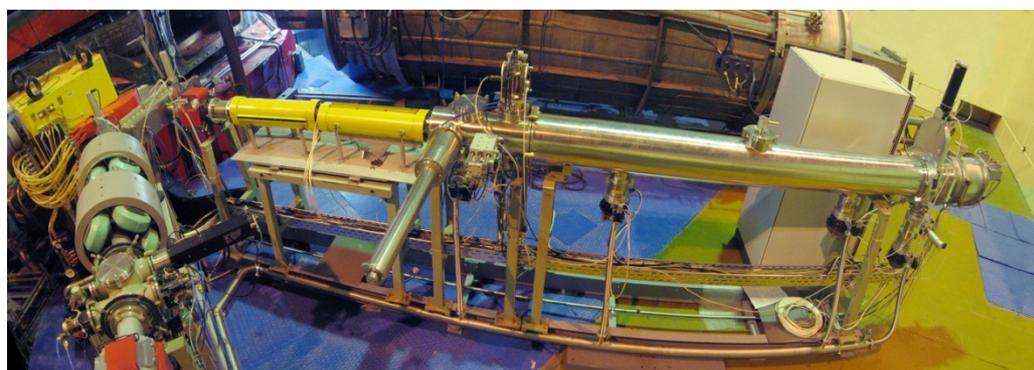
*FIG. C-1. Development of a new ion beam line for radiation hardness testing of electronic devices at the U400M cyclotron facility in the Joint Institute for Nuclear Research (Russian Federation).*
