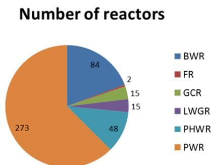
*FIG. A-3. Current distribution of reactor types. (BWR: boiling water reactor; FR: fast reactor; GCR: gas cooled reactor; LWGR: light water cooled, graphite moderated reactor; PHWR: pressurized heavy water reactor; PWR: pressurized water reactor).*
