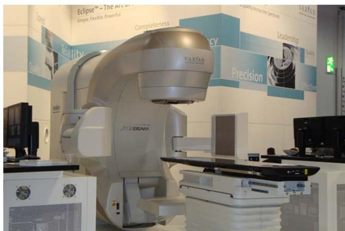
*FIG. E-1. A modern medical linear accelerator equipped for IGRT. This device enables increased radiotherapy precision by frequently imaging the target and/or healthy tissues just before treatment and acting on these images to adapt the radiation target. Photo: Eduardo Rosenblatt. ESTRO Forum, London 2011.*
