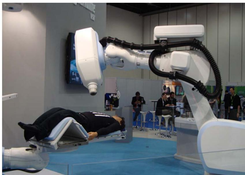
*FIG. E-2. Robotic radiotherapy is a frameless robotic radiosurgery system. The two main elements of this device are the radiation produced from a small linear accelerator and a robotic arm which allows the energy to be directed at any part of the body from any direction. Photo: Eduardo Rosenblatt. ESTRO Forum London 2011.*
