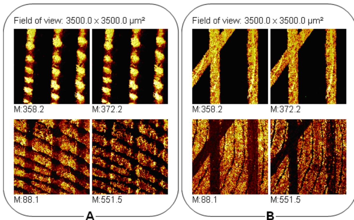
FIG. C-2. Positive ion images by keV ToF-SIMS of a fingerprint deposited (A) after ink and (B) before ink on a paper substrate. N.J. Bright, R.P. Webb, S. Bleay, S. Hinder, N.I. Ward, J.F. Watts, K.J. Kirkby & M.J. Bailey, *Analytical Chemistry*, 84(9), 4083–4087, (2012).
