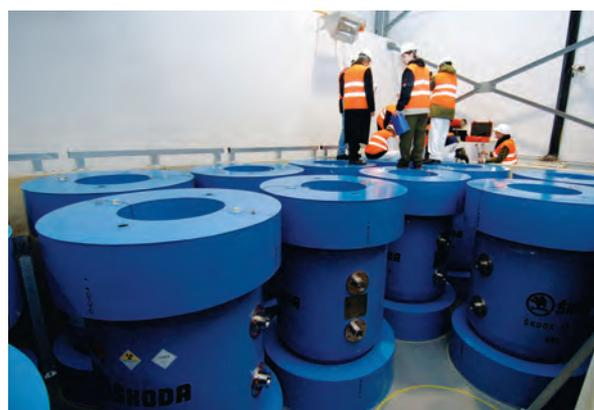
FIG. 1. Transport packages for radiation sources under preparation.
