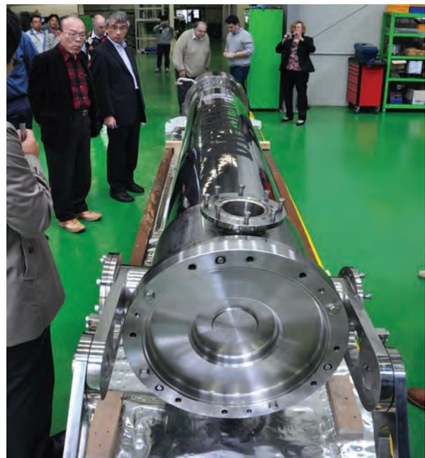
FIG. 3. Participants in the SPAR CRP inspecting the DrySim6 dry storage simulation test equipment at the Korea Atomic Energy Research Institute. (Photograph courtesy of VUJE.)
