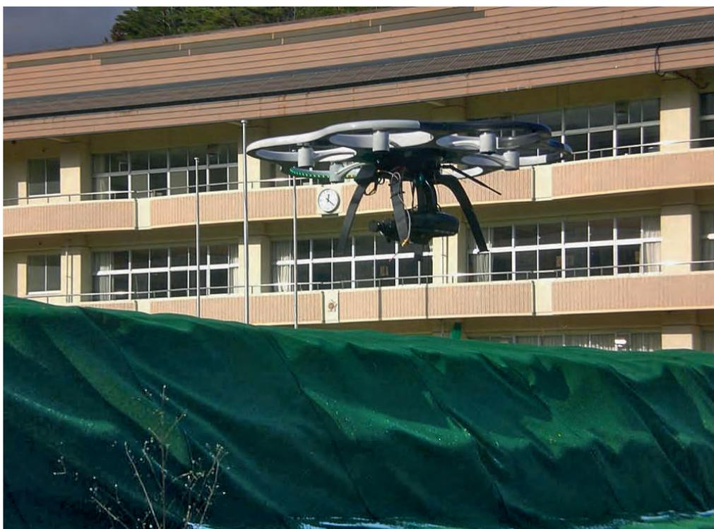
*FIG. 3. An Aibotix X6 UAV hovering over a temporary storage site in Fukushima Prefecture in December.*
