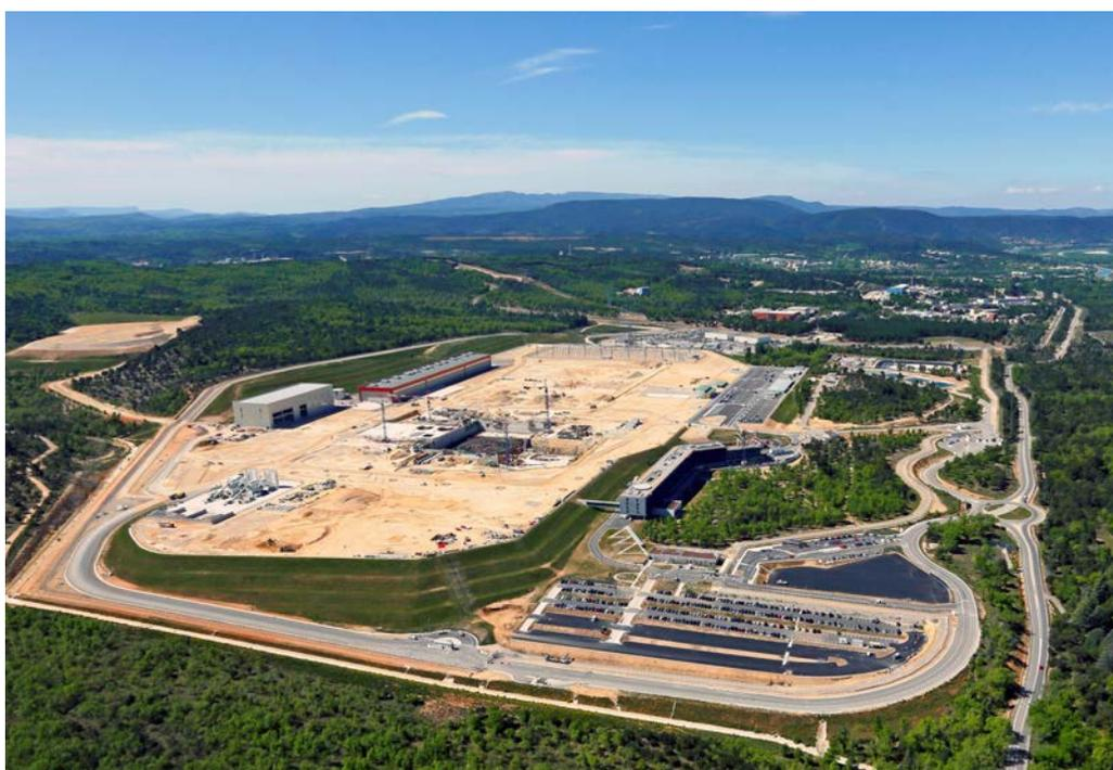
FIG. 4. Aerial view of the 42 hectare ITER platform at the end of 2014, with visible progress in the construction of office and functional buildings. (Photograph courtesy of ITER.)
