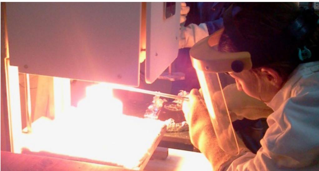
ARG/9/013: Melting glass in an electrical furnace as part of research into safe radioactive waste disposal, Nuclear Materials Laboratory, Bariloche Atomic Centre. Photo: CNEA.
