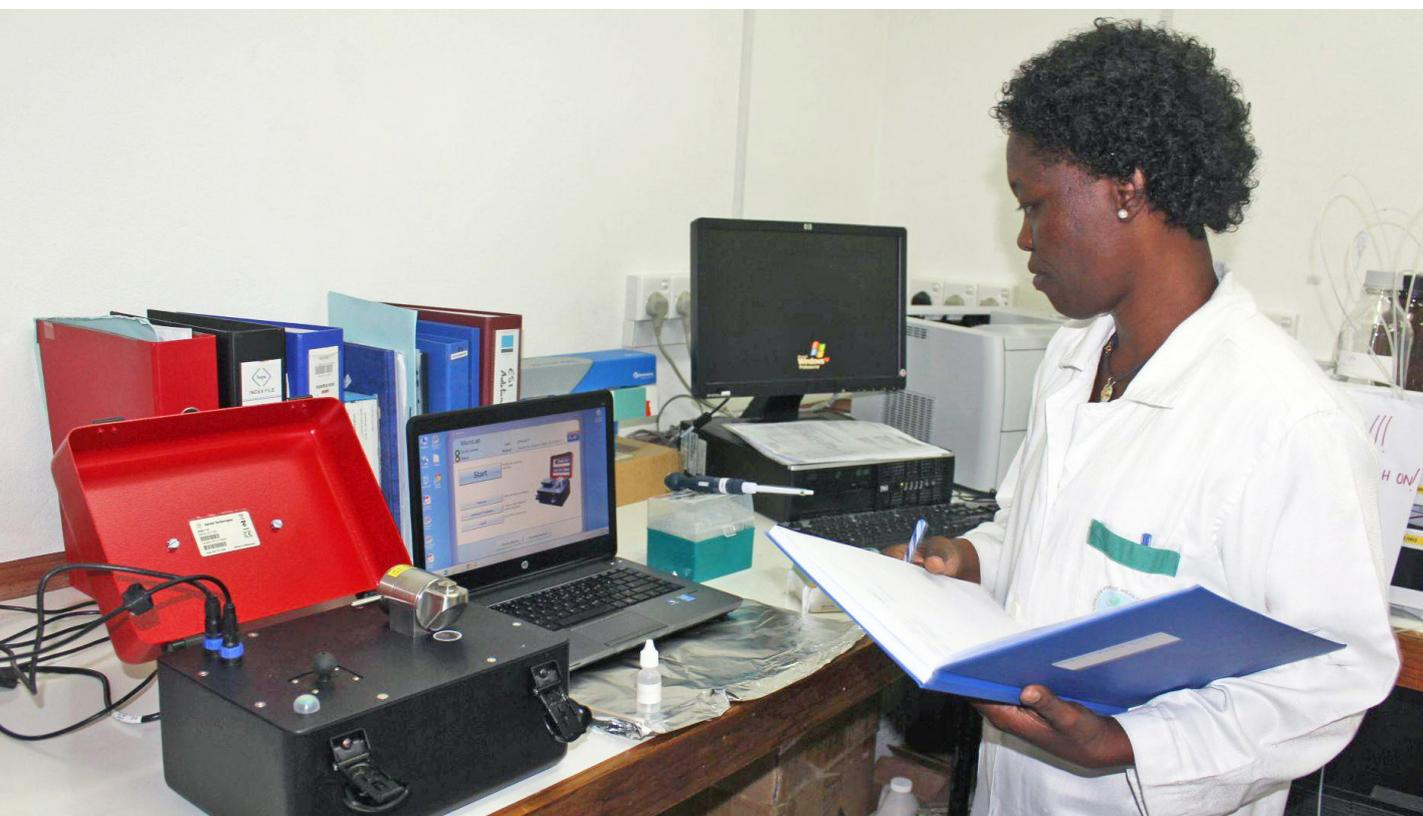
SEY/6/003: Analysis of deuterium enrichment by Fourier transform infrared spectrometry.
