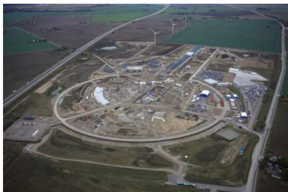
FIG. C-3. The European Spallation Source site in Lund, Sweden, as of October 2016. Fed by a pulsed 2 GeV proton linac delivering 5 MW average beam power, the world's most powerful neutron source is to start up in 2019 (Source: [https://dam.esss.lu.se/asset-bank/images/assets/33/40\\_2S5D41851.jpg](https://dam.esss.lu.se/asset-bank/images/assets/33/40_2S5D41851.jpg)).
