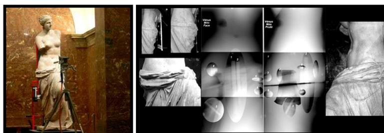
*FIG. H-4. Gamma radiograph showing the internal structure of the Venus de Milo statue in the Louvre Museum, France, used for decision-making before transporting. (Photos: IAEA)*
