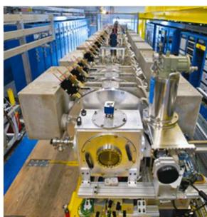
FIG. C-1. The NDCX-II accelerator<sup>12</sup> at the Lawrence Berkeley National Laboratory, Berkeley, USA, enables the study of structural dynamics in materials. The photograph shows the ten-metre long accelerator with the target end station in the foreground (Photo: Berkeley Lab).
