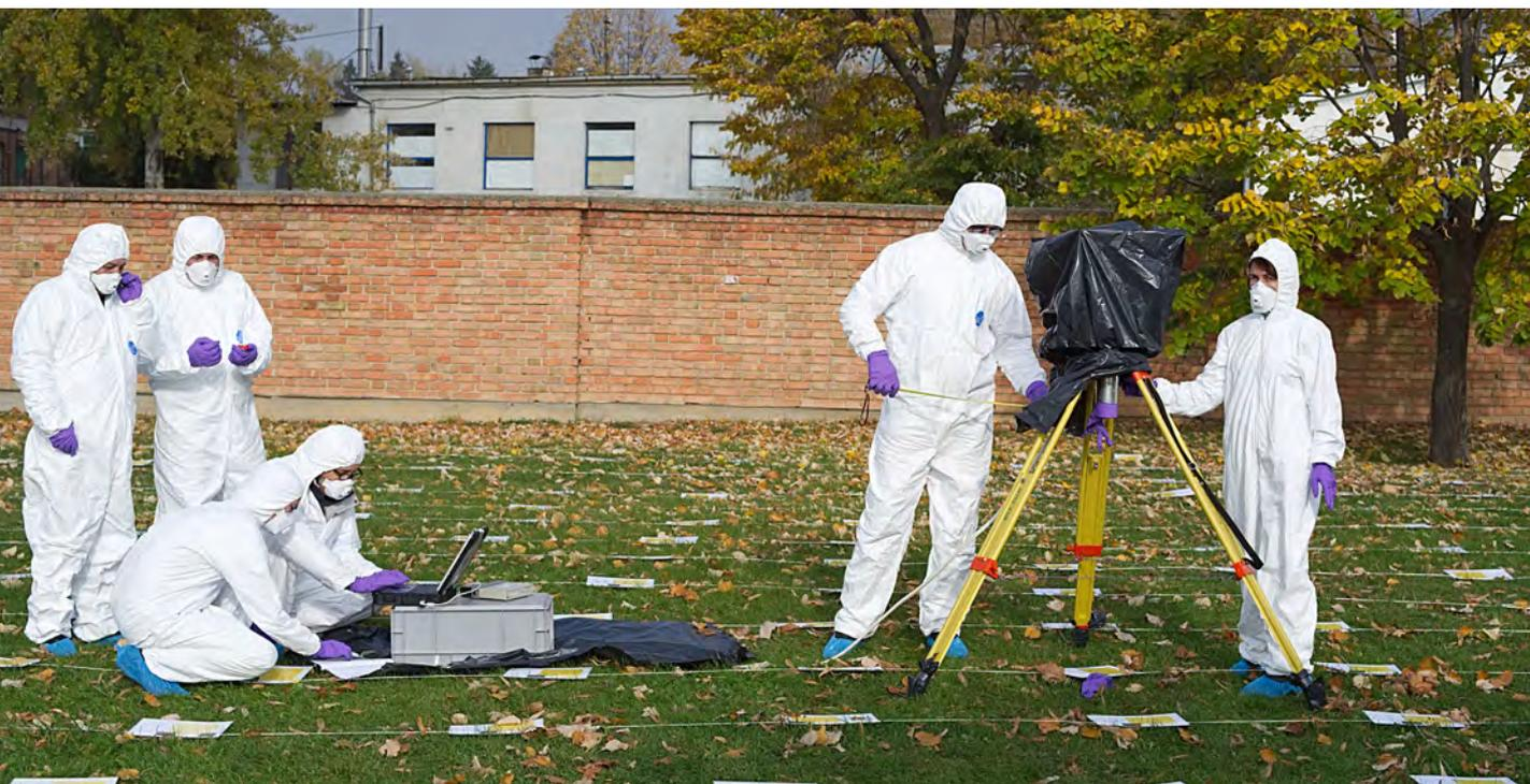
RER7008: Installation of an in-situ gamma ray spectrometer on a simulated contaminated site. Photo: S.Tarjan/IAEA.
