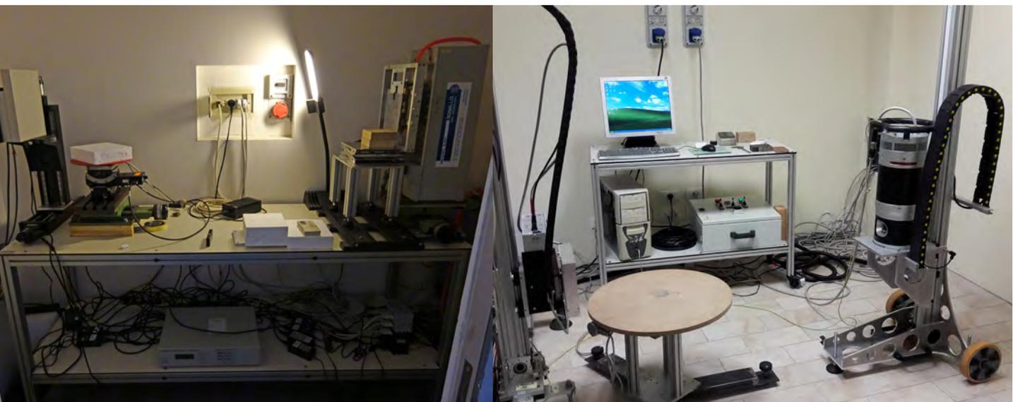
MAT0002: CT imaging, with the medium sized CT system (left) and the CT system used for large objects (right). Photos: M.Grima/Heritage Malta.
