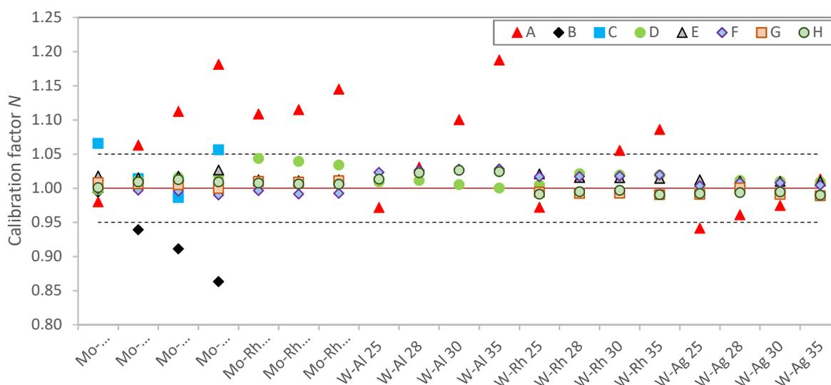
FIG. E-1. Calibration factor  $N$  (mGy/mGy) measured at the Agency's Dosimetry Laboratory for eight semiconductor based dosimeters (A–H) as a function of radiation quality.
