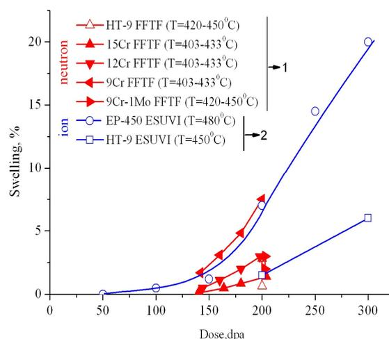
FIG. C-2. Comparison of materials swelling due to fast neutron (in red) and ion beam (in blue) irradiations, presented as a function of different damage doses (dpa: displacements per atom). (Courtesy of V. Voevodin, Kharkov Institute of Physics and Technology)
