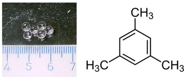
FIG. C-5. Image of pellets made at JINR-Dubna and used to moderate fast neutrons (left), and the schematic representation of their molecular structure. (Courtesy of JINR Dubna.)
