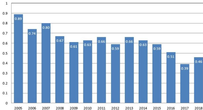
FIG. A-2. Mean rate of scrams: the number of automatic and manual scrams per 7000 hours of operation of a unit. (Source: IAEA Power Reactor Information System [www.iaea.org/pris](http://www.iaea.org/pris))
