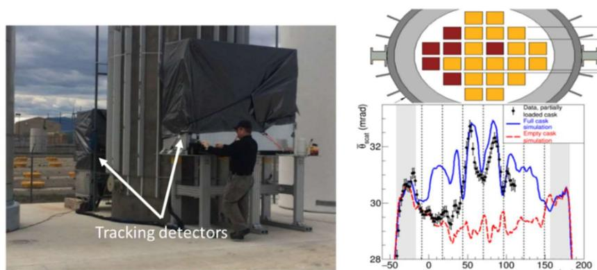
FIG. D-3. Photograph of muon trackers placed on two sides of a partially loaded MC-1 storage cask (left). A schematic showing the location of missing (red) and loaded (yellow) fuel bundles (top right). Experimental signal (black) compared to Monte Carlo expectations of a fully loaded (blue) and empty (red) cask (bottom right). (Photo: Christopher Morris, Los Alamos National Laboratory, USA).
