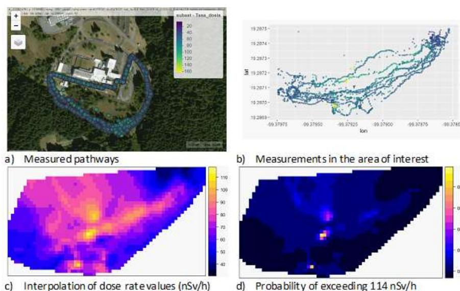
FIG. C-4. Example of the results of a field measurement exercise conducted as part of a national training course under TC project MEX7011. The measurement pathways are represented in maps, including interpolation of dose rates over the surveyed area as well as probability estimates for exceeding a given level. (Source: IAEA)
