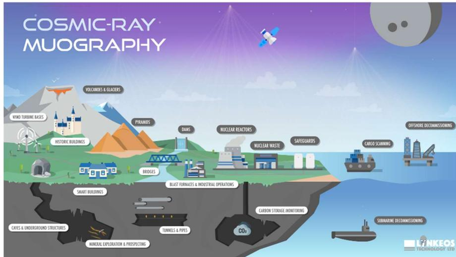
FIG. D-1. Schematic infographic illustrating the various applications of muon tomography (Source: Lynkeos Technology Ltd., UK)
