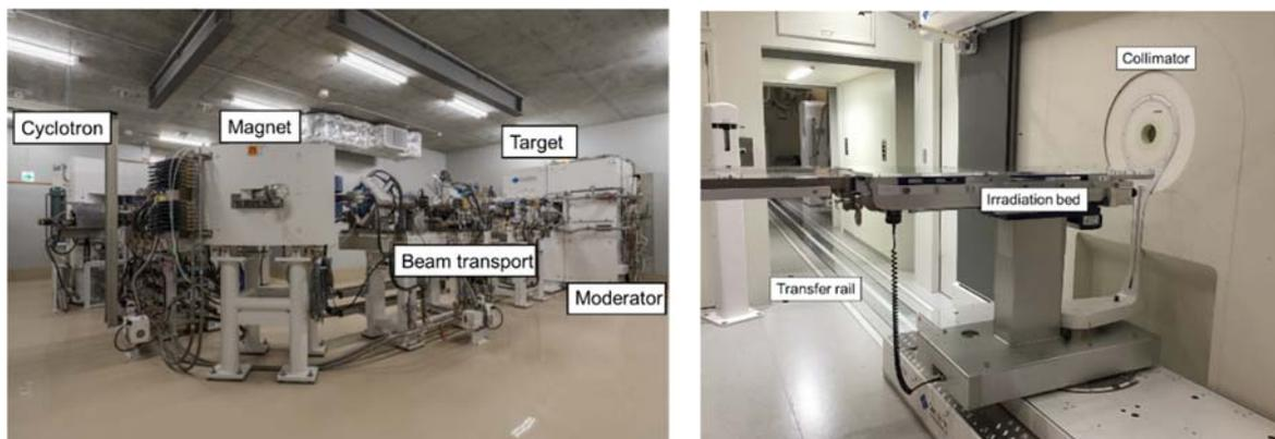
FIG. D-3. Accelerator and target components (left) together with patient irradiation position (right) at an accelerator-based BNCT centre. (Photos: Kansai BNCT Medical Center, Japan).
