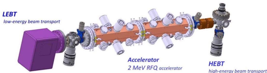
FIG. C-2. Schematic drawing of the main components of MACHINA. The ion beam can be extracted on the high-energy side of the accelerator to analyze the artifact. The very first applications are based on the PIXE technique, where X-rays are generated owing to particle-matter interactions. The emitted X-rays are then detected and, after data evaluation, the sample composition is determined.
