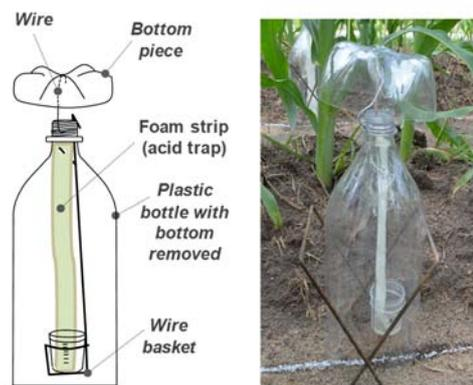
FIG. F-7: A view of the simple open chamber used to measure  $\text{NH}_3$  volatilization. Details of this chamber were described by Araújo et al. (2009)<sup>29</sup> and Jantalia et al. (2012)<sup>30</sup>.
