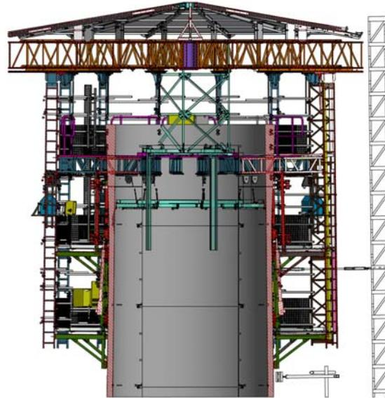
*Fig. A-11. Self-climbing platform designed to assist in the demolition of the ventilation stack of a legacy reprocessing plant at the Sellafield site. (Photo: Sellafield Ltd)*
