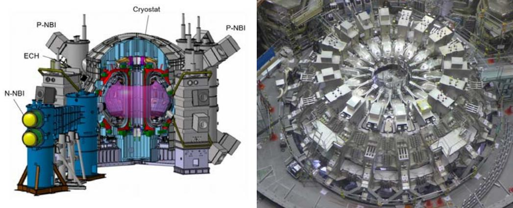
FIG. B-8. Schematic representation of the JT-60SA (left) with a photo of the close-to-completion torus assembly. (Source: P. Barabaschi et al., presented at the 2018 IAEA Fusion Energy Conference)
