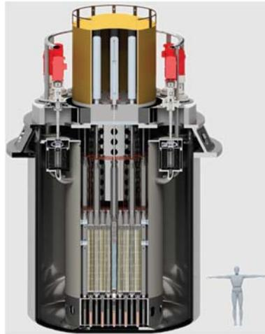
*FIG. B-5. 55 MW(e) SEALER-UK LFR design.*
