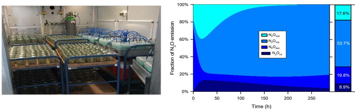
FIG. F-6: Laboratory incubation setup of a  $^{15}\text{N}$  tracing study (left) and results from a  $^{15}\text{N}$  tracing study to identify the  $\text{N}_2\text{O}$  emissions pathways from a permanent grassland;  $\text{N}_2\text{O}_{\text{nit}}$  = nitrification,  $\text{N}_2\text{O}_{\text{den}}$  = denitrification,  $\text{N}_2\text{O}_{\text{org}}$  = heterotrophic nitrification,  $\text{N}_2\text{O}_{\text{cod}}$  = codenitrification.
