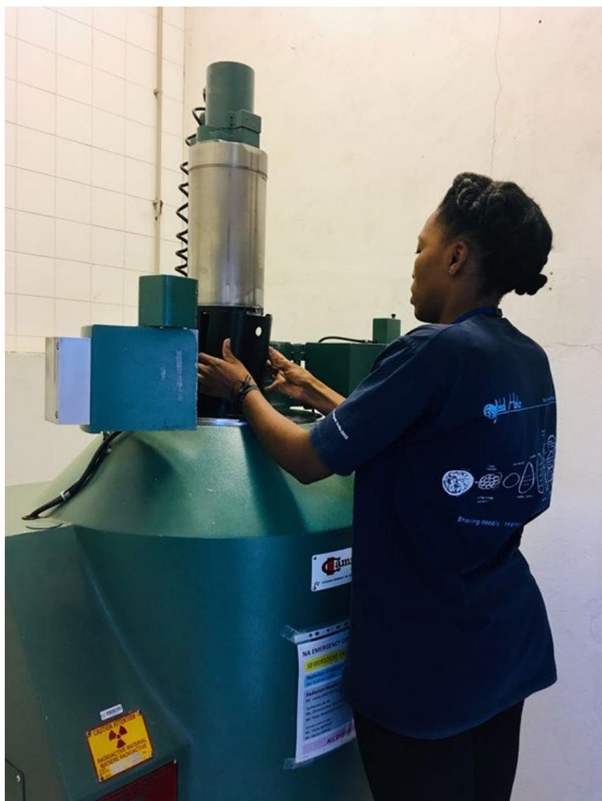
FIG. B.1. Male mosquitoes are loaded into the chamber of a Gammacell 220 unit for sterilization.
