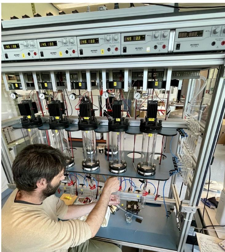
*FIG. B.1. New method for tritium enrichment based on permeable electrolytic membrane technology.
