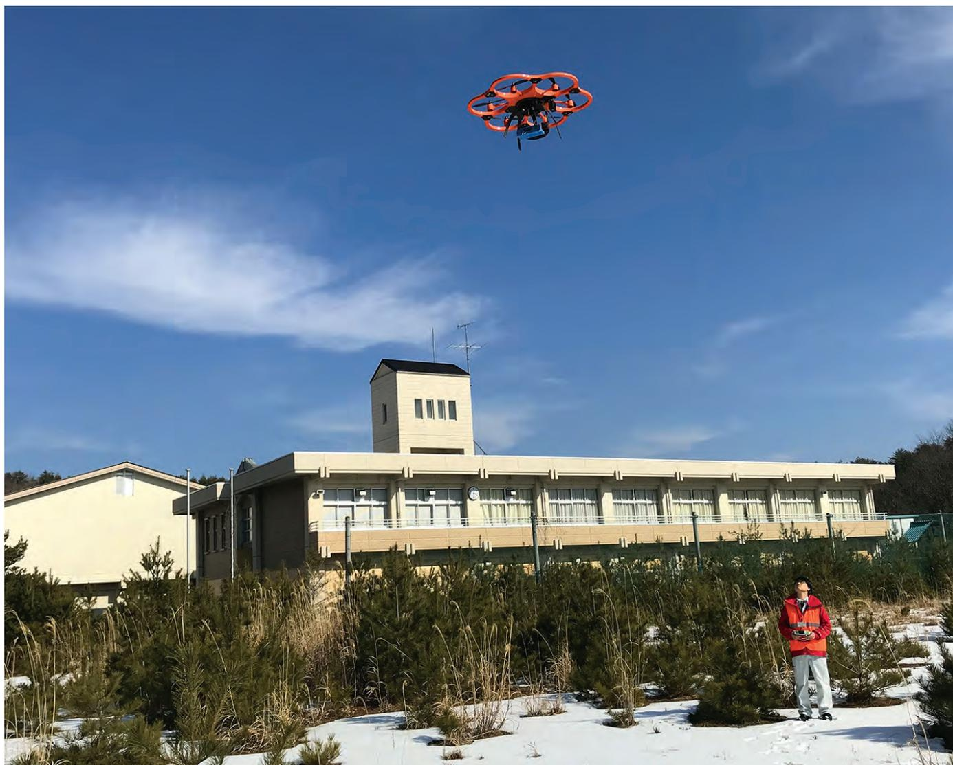
FIG. 3. A new technology using drones, developed by the Agency for use by the authorities of Fukushima Prefecture, Japan, allows for radiological measurements. (Photograph courtesy of Fukushima Prefecture.)
