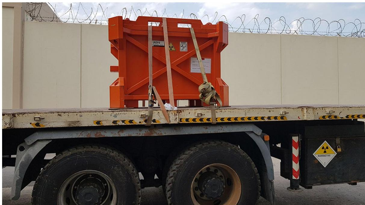
*The disused sealed radioactive source packed in the licensed container ready for international transport. (Photo: IAEA Contractor)*
