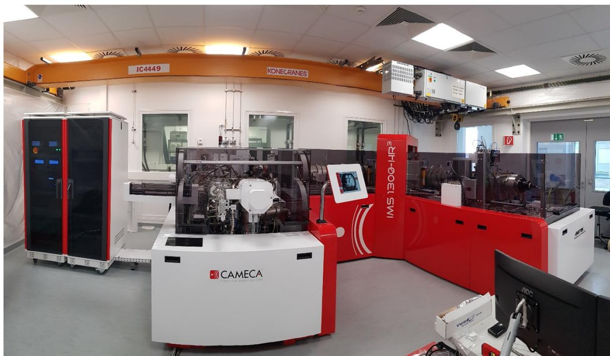
*The new Large Geometry Secondary Ion Mass Spectrometer (LG-SIMS)
