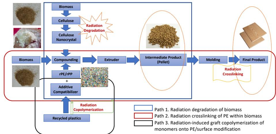
FIG. F-2. Scheme of the proposed production steps for reinforced wood–plastic composite with natural fibres and recycled plastics (recycled polyethylene and recycled polypropylene, rPE/rPP). (Image: National Nuclear Energy Agency of Indonesia)
