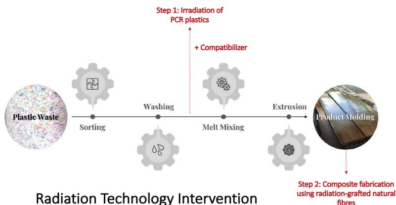
FIG. F-1. Scheme of the proposed composite fabrication using radiation-grafted natural fibres and irradiated post-consumer recycled (PCR) plastics in the Philippines. (Image: Philippine Nuclear Research Institute)
