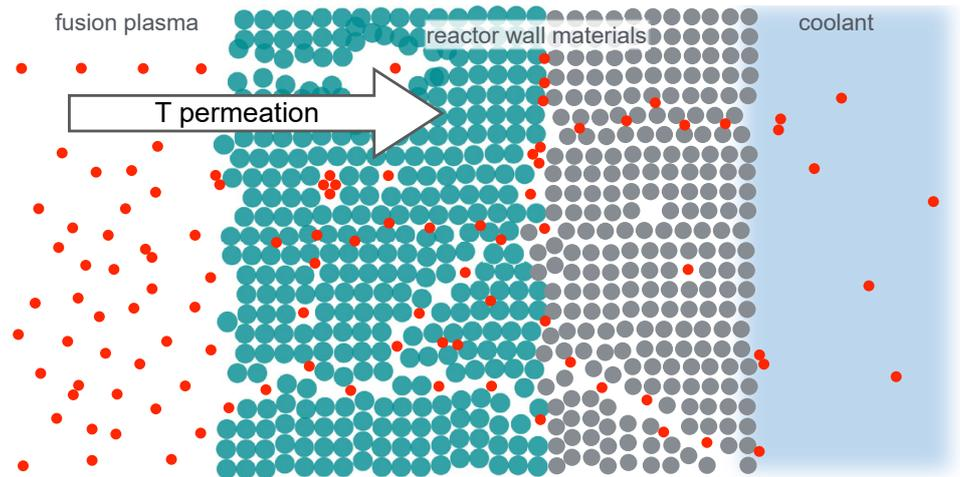
FIG. E-1. Schematic display of the tritium permeation process in a fusion reactor wall.
