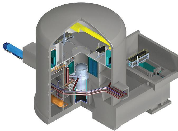
FIG. A-6. Canadian SCWR design — cutaway view of reactor building. (Image: Schulenberg and Leung, Canadian Nuclear Laboratories)
