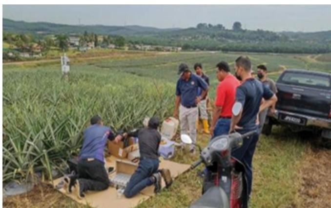
Installation, calibration and validation of cosmic ray neutron sensor at Kulim Pineapple Farm. (Photo: Selangor Study Site)
