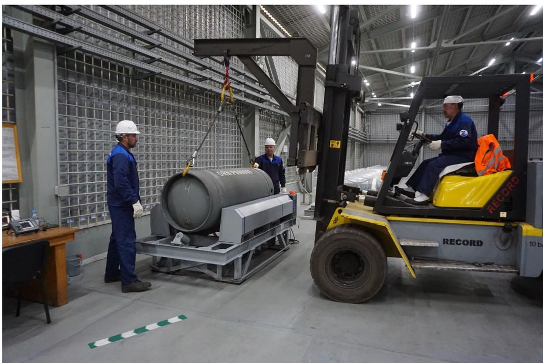
*FIG. B.3. Recertification of the LEU-filled 30B cylinders at the IAEA LEU Bank.*
