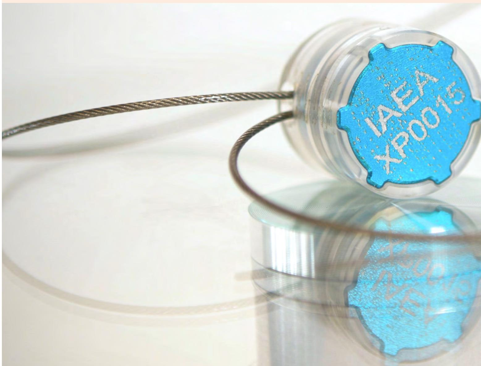
The result is a state-of-the-art seal made from aluminium and polycarbonate, unlike the traditional seal, which was made from copper and brass. The new seal requires no tools to apply, no maintenance while deployed and no batteries. Its components have unique features and pattern designs etched into their surfaces that cannot be replicated without detection. This makes the new seal even more secure and enables the verification and reporting carried out by inspectors to be streamlined.
