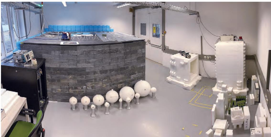
*After full commissioning of the Agency's Neutron Science Facility, shielding structures housing deuterium–deuterium (right) and deuterium–tritium (left) neutron generators were employed to deliver the first two-week hands-on training course on neutron science and applications.*
