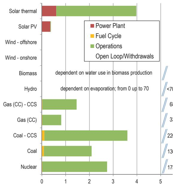
Fig. 8. Life cycle water consumption (in m<sup>3</sup>/MW-h) for electricity technologies.<sup>13</sup> Water used in operations (dark green) refers to cooling towers, while light green shows water withdrawals for the alternative of once-through cooling.
