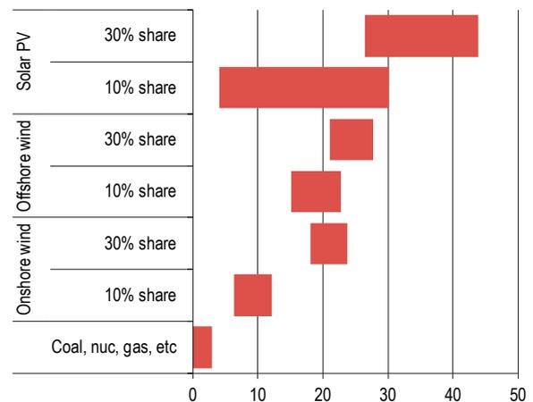
Fig. 5. Illustrative system costs in US \$/MW·h (including backup, balancing and grid).<sup>8-10</sup> Estimates are highly system and site specific, with costs potentially higher for specific configurations, or lower where there is excess capacity.
