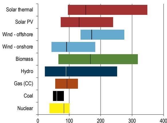
Fig. 4. Levelized costs of electricity generation (US \$<sub>2013</sub>/MW·h) at 7% market discount rate.<sup>8,9</sup> Bars indicate low, median and high estimates.
