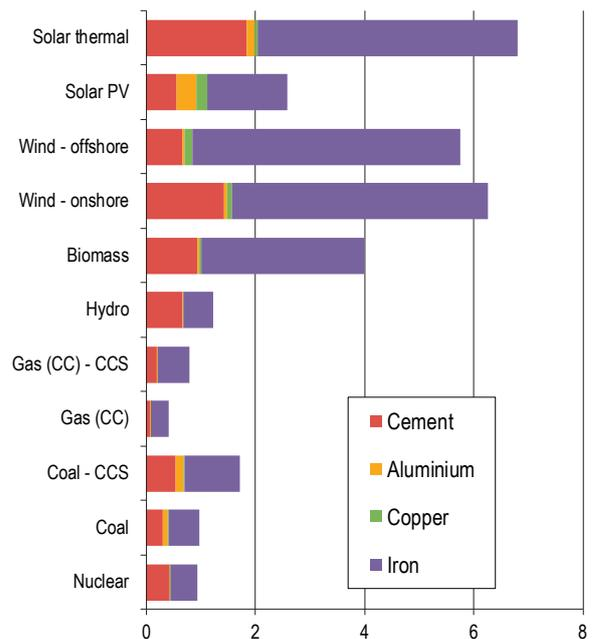
Fig. 10. Life cycle structural material requirements (g/kW-h) for electricity technologies, 2010 global average.<sup>9, 11</sup>
