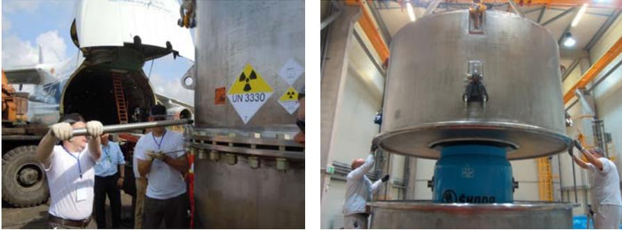
*FIG. C.5. Tightening the bolts on special transport packages carrying spent HEU fuel from Viet Nam's Dalat Nuclear Research Institute to the Russian Federation (left). Placing a protective overpack on a transport cask containing spent HEU fuel from the BRR in Hungary (right). This overpack was designed to permit air transport.*
