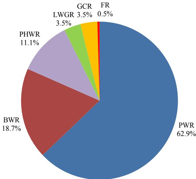
**Note:** BWR — boiling water reactor; FR — fast reactor; GCR — gas cooled reactor; LWGR — light water cooled, graphite moderated reactor; PHWR — pressurized heavy water reactor; PWR — pressurized water reactor.
