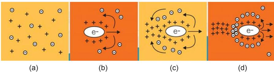
**Note:** (a) Positive ions and free electrons forming a plasma. (b) An electron bunch enters the plasma and repels all free electrons. Positive ions are attracted around the bunch. (c) The already displaced free electrons are now attracted by the positive ions left behind the bunch. (d) The free electrons in their new position behind the bunch accelerate the electron bunch.
