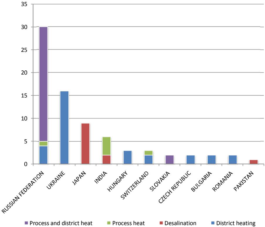
FIG. A.6. Number of reactors used for both non-electric purposes and electricity production.
