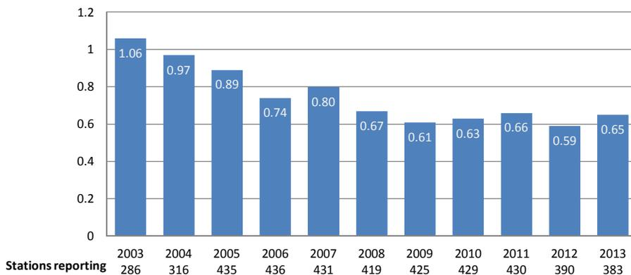
FIG. A.16. Mean rate of scrams: The number of automatic and manual scrams that occur per 7000 hours of operation.
