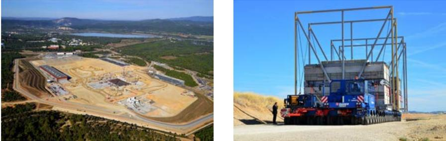
*FIG. B.4. The ITER site as of September 2013 (left). The 800 t trailer with remote controlled vehicle, replicating the weight and dimensions of the largest ITER loads (10 m tall, 33 m long and 9 m wide), travelled at an average speed of 5 km/h for four consecutive nights to test the 104 km long ‘special itinerary’ (right) (courtesy of ITER).*
