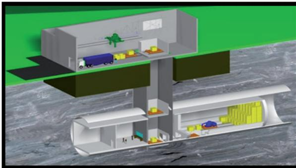
FIG. A.15. Concept of emplacement operations at the Russian Federation's planned LLW disposal facility (courtesy of the All-Russia Design and Research Institute for Integrated Power Technology).
