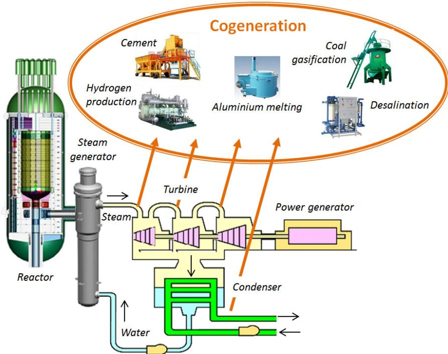
FIG. B.3. Schematic representation of cogeneration.
