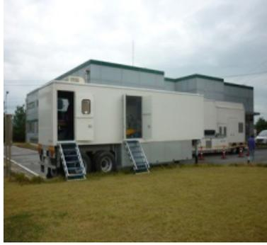
*FIG. F.2. A mobile electron beam accelerator installed in sewage treatment plant (courtesy of KAERI).*
