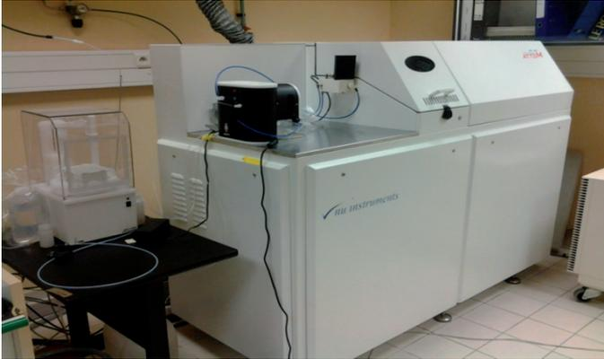
*FIG. H.2. High resolution inductively coupled plasma mass spectrometer used to analyse stable lead isotopes in environmental samples.*
