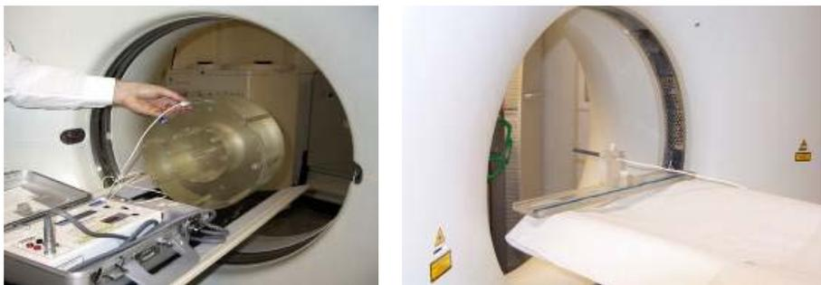
*FIG. E.1. Measurement of dose in CT in a standard polymethyl methacrylate body phantom, and in air.*
