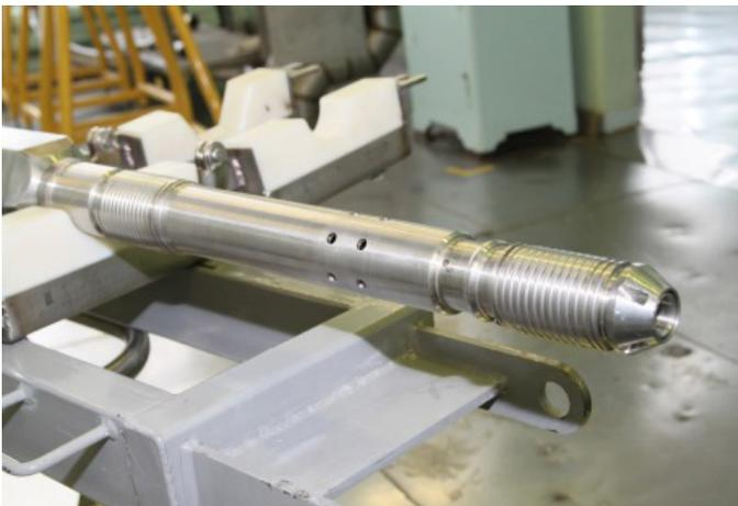
*FIG. A.7. TVS-5 fuel assembly, the prototype fuel for the advanced BREST-300 reactor. (Photograph courtesy of SCC.)*
