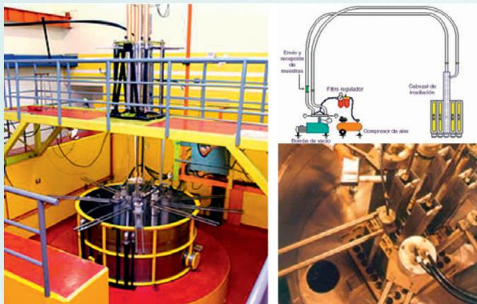
RP-0 top showing bridge mechanisms (left), pneumatic delivery system, control rods and neutron detectors (right).
